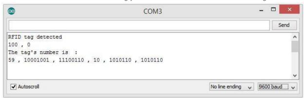
When the RFID reader senses a card, it starts by printing "RFID tag detected" on the Serial Monitor. The next line verifies the card type. In normal use, this would be unnecessary. The next two lines print out the data stored in the card, in this case an ID identifying the specific tag scanned.
