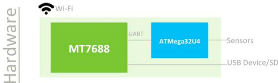
Figure 52 Smart 7688 Duo Hardware Architecture
