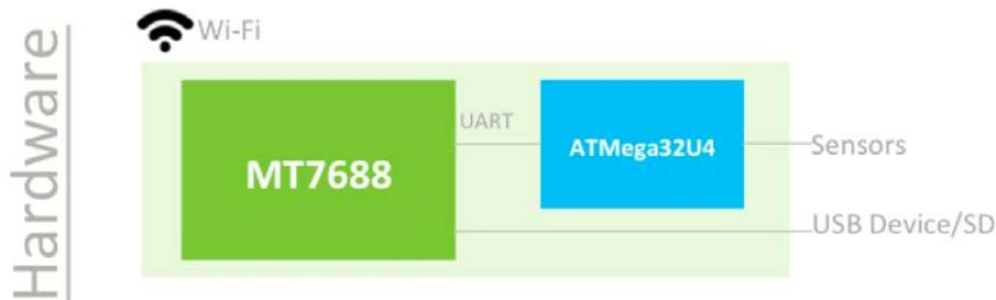
Figure 44 LinkIt Smart 7688 Duo Hardware Architecture
