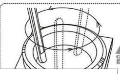
3, Melting Stannum: it takes around 10 minutes for totally melting. Caution: Must melt the stannum rod along the inside surface of the pot at the first time, melt it in the air is not allowed
