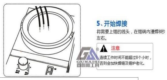
5, Start welding: soak the head of the wire into the pot for 8 seconds or so, Caution: the total time cannot be over 8 hours for constant working, otherwise, the pot might be getting aged sooner
