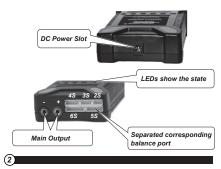
Connect the proper Lipo battery( 2~6 cells) with charger as following:
