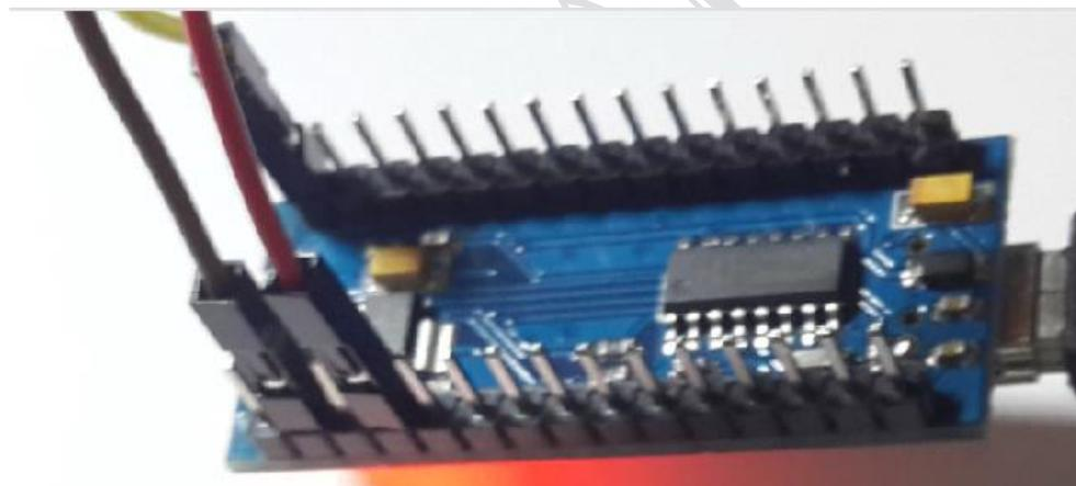
Note: MCU (TX) - Serial port TX or RX need to see the serial port of the screen model, the serial port is reversed just does not work, so when it does not work, try to take another line;
