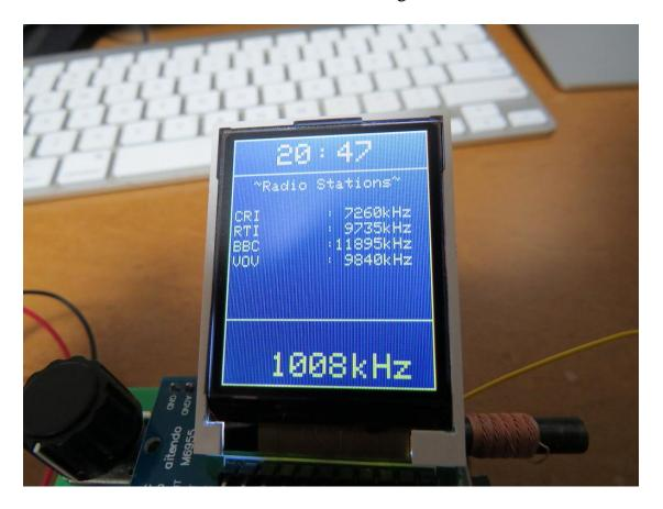
Bar antenna is out of the Yokotcho because it significantly performance degradation and put under the DSP radio module (in a state, such as placing the antenna in the shield).
