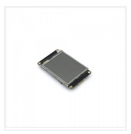
Nextion Enhanced NX3224K028 is a powerful 2.8" HMI TFT Touch Display, with 16MB Flash data storage space, 1024 byte EEPROM, 3584 byte RAM, and GPIO supported.
