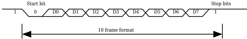
Frame format for transmission: 1 level start bit, 8 bit data (LSB first) and one stop bit, no parity bit.
