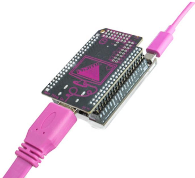
The HDMI DIP is extremely easy to use. Once you have your C.H.I.P. OS updated, it's really as simple as attaching the DIP to your C.H.I.P., plugging in an HDMI monitor, plugging into your power supply and booting up C.H.I.P. But, for posterity's sake, here's all the details.
