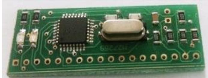
Because the decoder stage of LRN60C is microcontroller based, an important feature is the Code Learning Capability. The module can learn 60 different-coded remote transmitters. So, there is no need for soldering any address pins nor using a hardware dip-switch for address matching with the transmitters. This is a key feature that LRN60C differs from ordinary remote decoder IC's.
