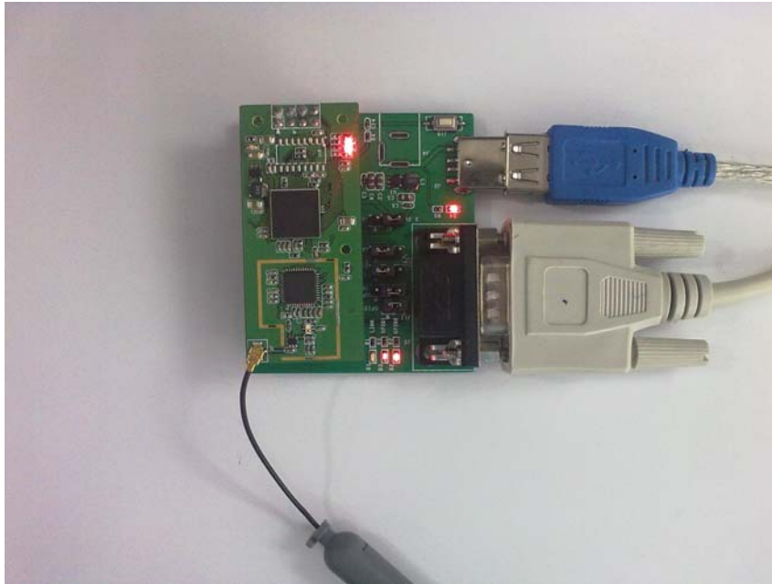
Figure 3-1 connection between with serial adapter board and UART-WIFI module
