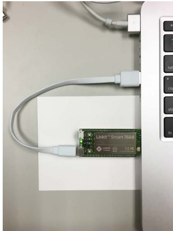
Figure 1 Providing power to the LinkIt Smart 7688 board
