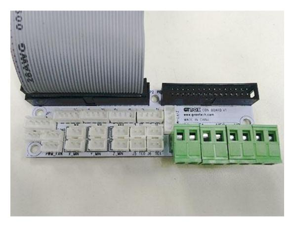
Step7. Connect the other end of the ribbon wire to the control box.
