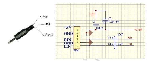
Module audio input and output ports, external 10uF capacitor, and then direct wire or solder stereo plug wiring. Module 5V DC power supply, can also be used directly to supply three AA batteries, the case of an external 5V switching power supply, the module port to add the decoupling capacitor 100uF the best positive power supply and then a series of inductors.
